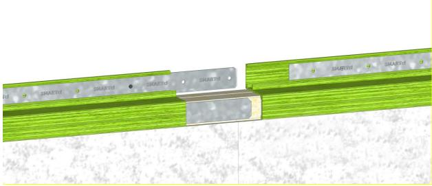
Steel inserts extend min. 3" with 1/16" to 3/16" gap for thermal expansion
