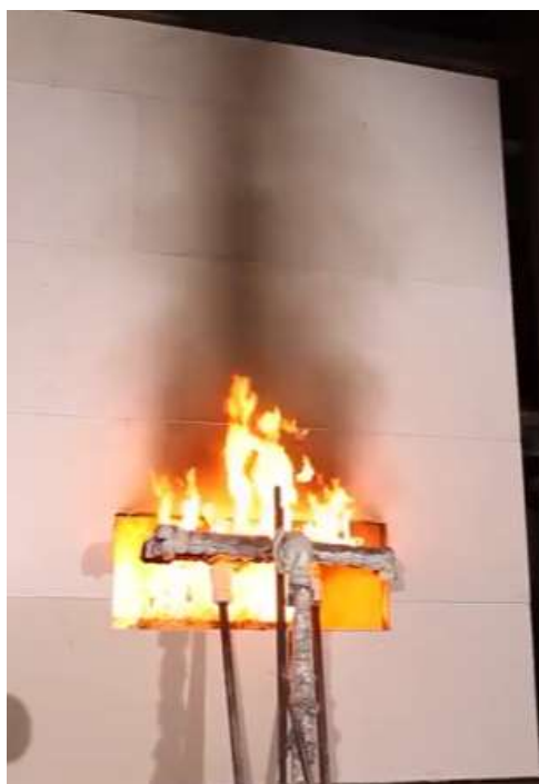
Figure 3: An NFPA 285 test is shown with a fire plume extending up the wall.
