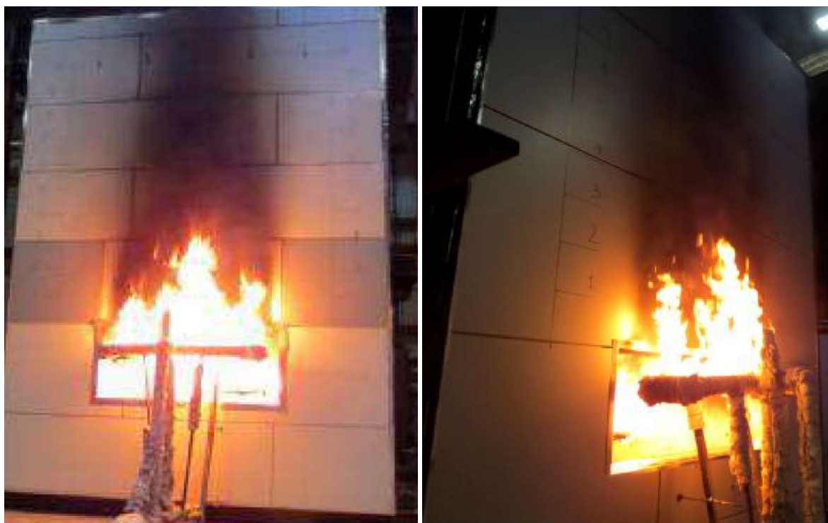
Figure 5: NFPA 285 testing with GreenGirt is shown.
