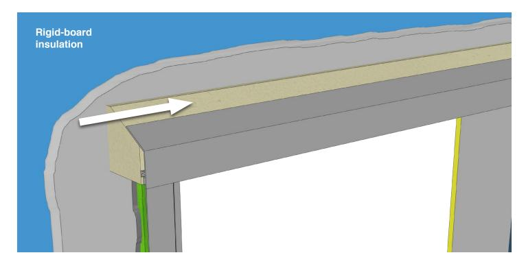
13. If using mineral wool insulation, cut the insulation header piece to fit on top of the header angle and behind the aluminum angle insert, then slide into place.
