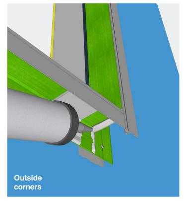
10. Use a sealant finishing tool to create a wide radius of sealant in each inside and outside corner.
