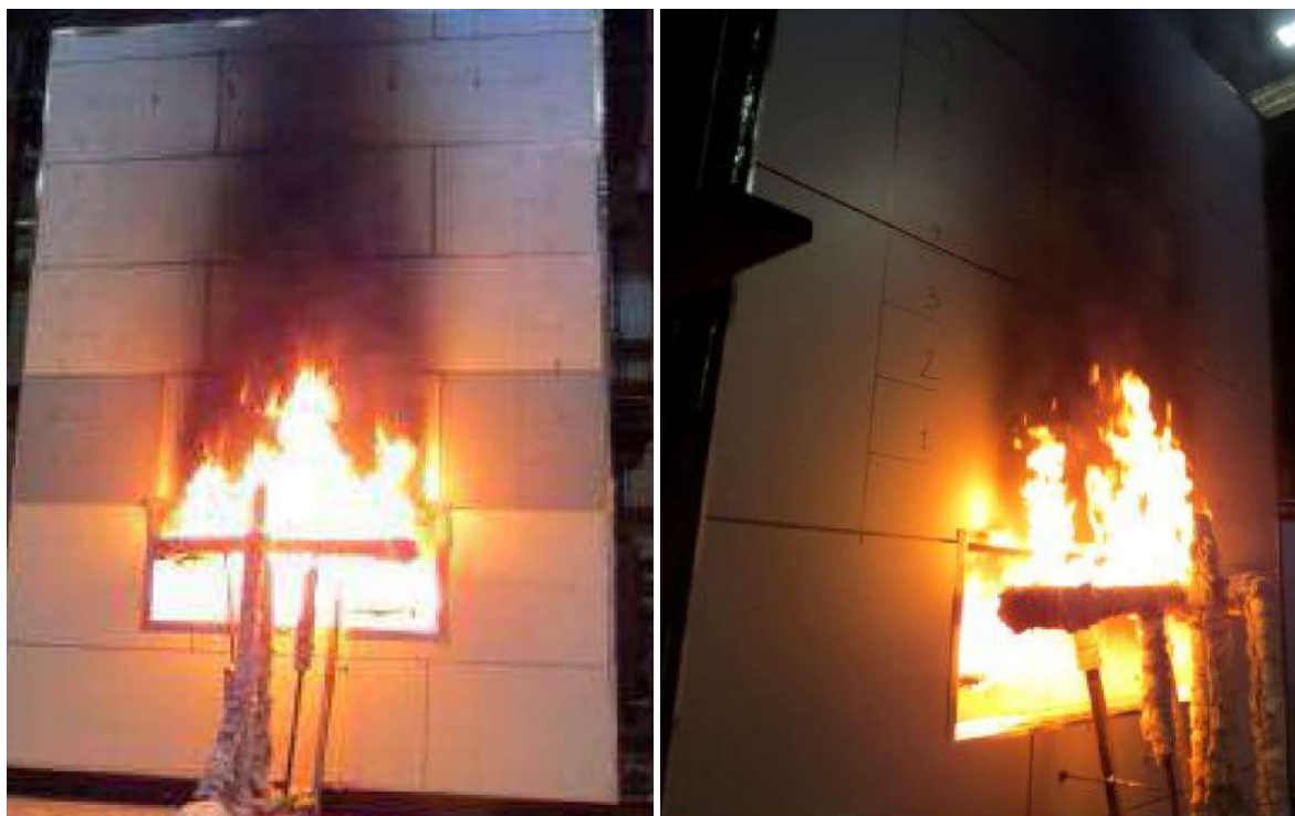
Figure 5: NFPA 285 testing with GreenGirt is shown.
